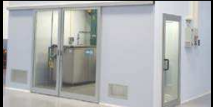
White room for assembly of hydraulic actuators critical parts
